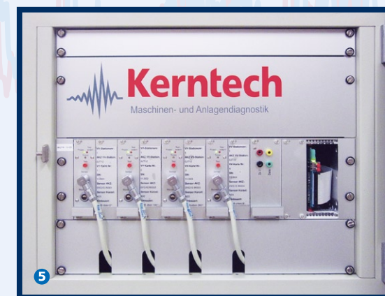
Fig. 5: Updated preamplifier rack: new amplifiers integrated into legacy system
