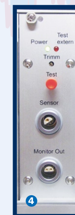
Fig. 4: Preamplifier with self test function
