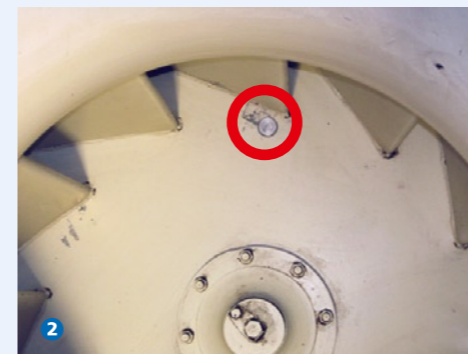
Fig. 2: Balanced fan with mounted balancing mass (red circle)
