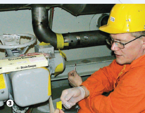
Fig. 1: Shock tests for the determination of solid borne sound in a nuclear power plant
